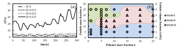
Fig. 2 (a) Time evolutions in stresses for different ethanol content at the shear rate of 10 s<sup>-1</sup>. (b) oscillation mode maps at  $\beta$ =0.035 for different contents of polymer and particle.
