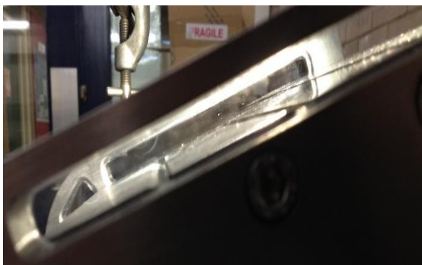
Fig.2: A view through the sapphire glass onto the slide with the slot exits being visible.
