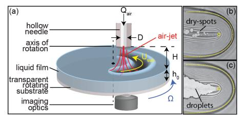
Fig. 1: (a) A schematic of the experimental setup. (b,c) Interference micrographs and numerical simulations (dashed lines) of a thin liquid film deformed and ruptured due to a moving air-jet for different experimental conditions.
