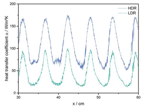
Figure 1 – Distribution of the heat transfer coefficient  $\alpha$   $W/m^2K$  as a function of the position in the dryer.
