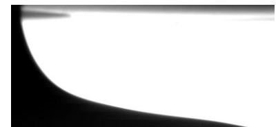
Fig. 2, HS-image of a cross sectional view of a receding tail at high scan velocity.
