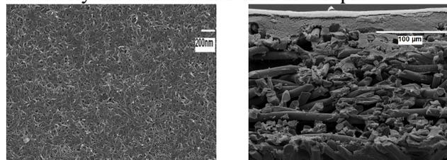
Fig.2 CNTs coated GDL (a) side view (b) cross view
