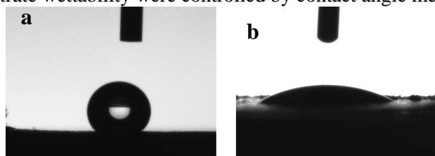
Fig. 1: Effect of surfactant on surface tension: (a) 5 $\mu$ l droplet of water without surfactant; and (b) 5 $\mu$ l droplet of CNTs/Tween 80 ink. The surfactant decreases clearly the surface tension of the droplet
