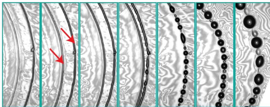
Fig. 2. Optical micrographs of an aliphatic thin liquid film on a rotating substrate ( $\Omega = 1$  rpm) at 1, 2, 3, 5, 9, 17 and 33 minutes after interaction with an atmospheric Ar plasma jet [1]. Image widths 4 mm.
