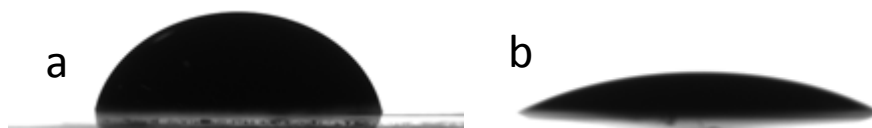
Fig. 1: Droplet of NMC532 slurry on Al foils (a) untreated Al foil and (b) corona treated Al foil.
