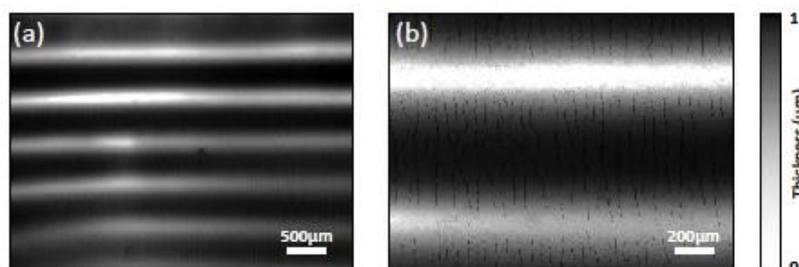
Fig. 2. (a) Latex dried film thickness oscillation. (b) Presence of regular fractures as thickness increases within the film.
