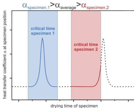
Figure 2 – Schematic drawing of HTC profiles for specimen dried at different positions within the same coating.
