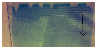
Fig. 2: Unstable coating resulting in barring.
