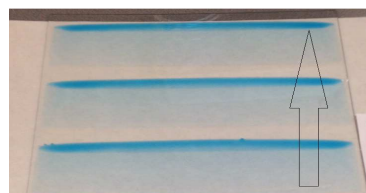
Fig. 1: Layer with large trailing edge and non-uniform coating.
