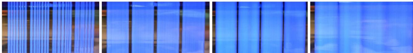
Picture 1.1 till 1.4 showing the change in the appearance of the stripes by increasing the volume flow
