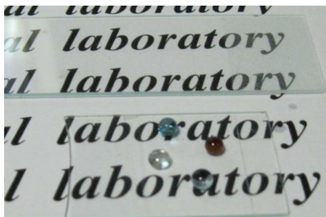
Fig. 1 Digital image of the S_5S'_2S''_3 coating with water (A), ethylene glycol (B), diiodomethane (C) and hexadecane (D) droplets on its surface.
